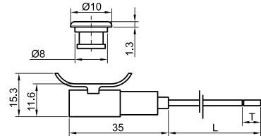
The lens connected from the front panel is fitted with the indicator body positioned on the back of the panel in correspondence with the drilling template (4 support points)
