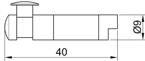
Light indicator with a device for quick connection
