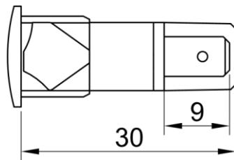
**Self-locking LED light indicator with front panel's connection and thin head (thickness 2,5mm)**
